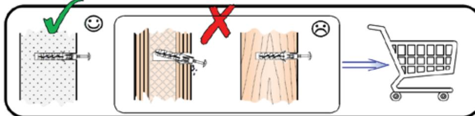
**-EN-** Before suspending or fixing furniture to the wall (in order to prevent falling over), check the type and strength of the wall. Select wall plugs and screws appropriate for the given type of the wall. In the case of doubts, contact a specialist. The installation must be performed by a competent person. **WARNING!!! If the rawplugs with screws are attached to the product, then they are intended only for walls made of solid and homogeneous materials.**
